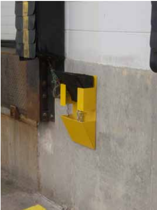
Wheel Chock Cradle, Chock and Chain in Use
